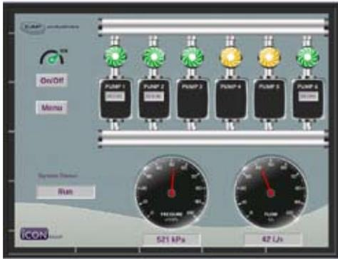
Key information including variable speed status, motor speed, system pressure & flow is clearly displayed on main screen (viewable via the internet).
